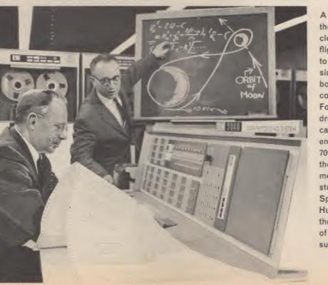
A principal target of the Saturn space vehicle is the execution of a flight around the moon to explore the other side of this heavenly body. The actual flights cost millions of dollars. For only several hundred dollars, a flight can be simulated mathematically on the IBM 7090 computer. Here, the calculation of a moon orbit is being studied at the Marshall Space Flight Center in Huntsville, Alabama. At the left is a model of Saturn's powerful super-booster.
